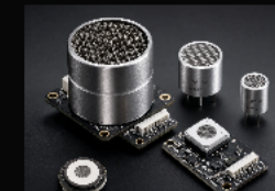
Gas Sensors O 2 / CO 2 / CH 4 / propane / ammonia
